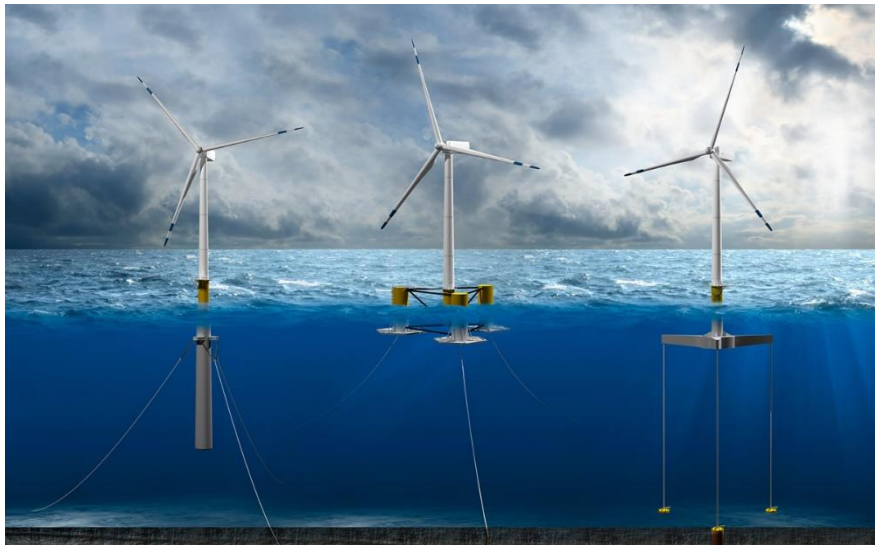
Three main types of floating offshore wind turbine. (left) Spar type, (middle) semi-submersible and (right) tension leg
