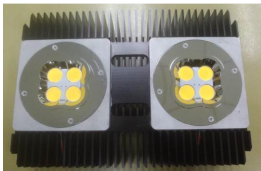
Development of modular ultra-high-power LED lamp technology (slim optical components and multi-layer low thermal resistance)
