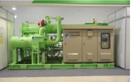
Establish paper made 125kW turbine ORC power generation system
