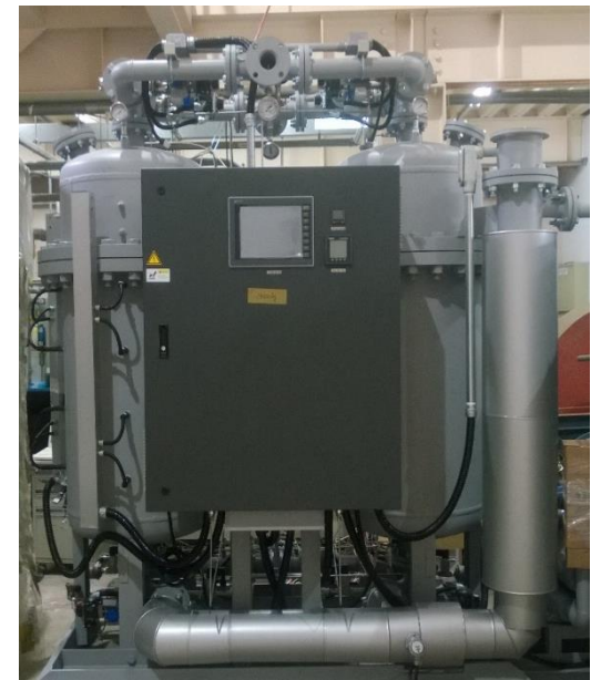
10CMM adsorption dryer with directly electric heating regeneration
