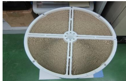
610mm dehumidification wheel with directly electric heating regeneration (commercial device)
