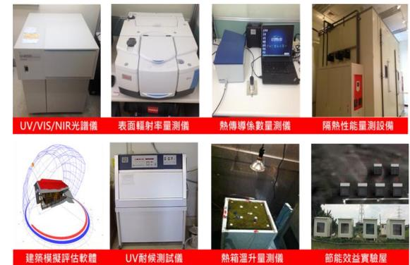
The testing equipments for building material energy-saving efficiency
