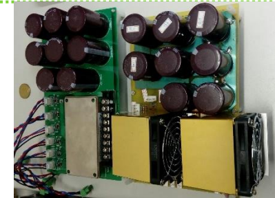
25 KVA community-based three-phase converter
