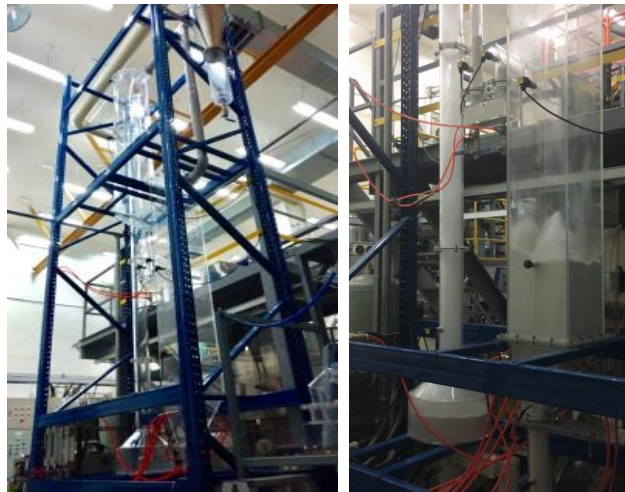
The Cold Mode of 100\text{kW}_{\text{th}} Indirect Fluidized-Bed Gasifier ( Left: Overall facility, Right: Experiment execution )
