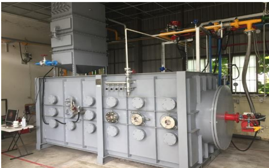
100 kW Gas Research Furnace
