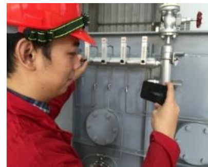
200 kW Fluidized Bed Research Furnace
