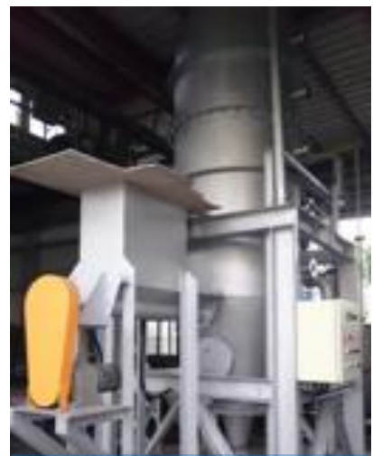
200 kW Fluidized Bed Research Furnace
