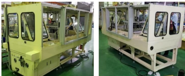
Photos of full-scale slot die coating machine for perovskite solar cell
