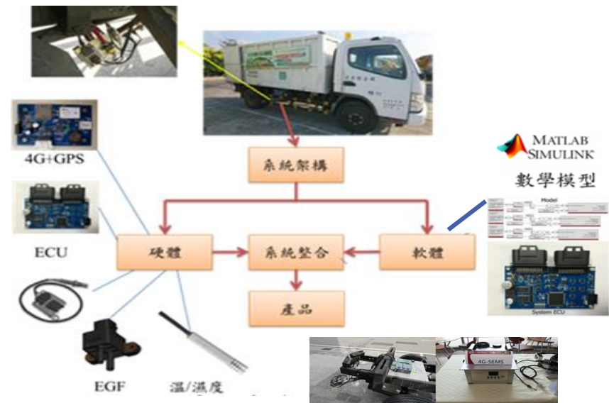
Simple Wireless Emissions Measurement System
