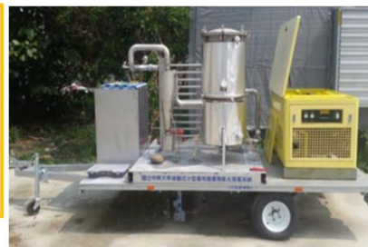
移動式小型農牧廢棄物氣化發電系統 Small-scale Mobile Gasification Power System for Agricultural Waste
